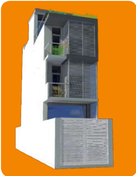
Variation of town house type with closed heat buffer zone (Source: Hesse 2011)
